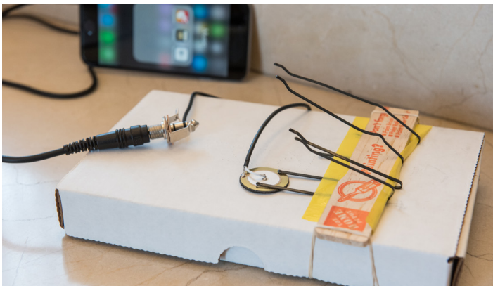
Piezoelectric pickups are simple transducers that can easily be added to many musical instrument crafts.
